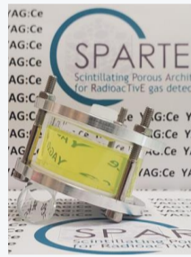
Inorganic porous scintillators
