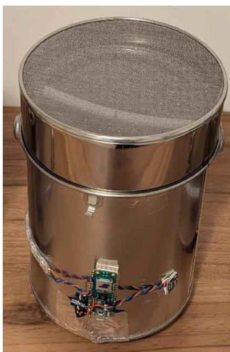
Low-cost LVIC Rn-222 detector
